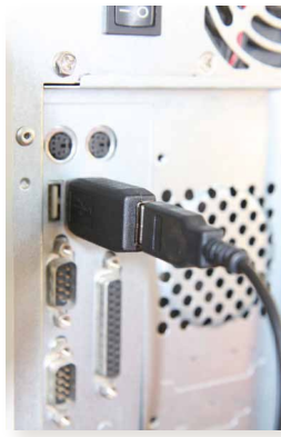
Figure 7. Key logger that collects all keystrokes.
